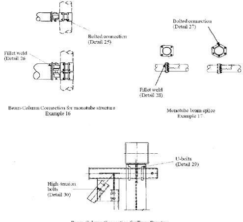
Beam-Cohunn Connection for Truss Structure Example 18
